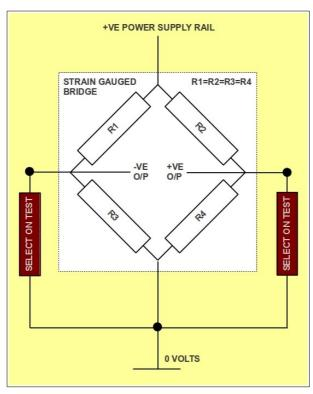
A supply of suitable resistors must be available. These must be metal film resistors (MF25 series) and a comprehensive range is required of preferred values between 100 ohms and 10 meg ohms.
